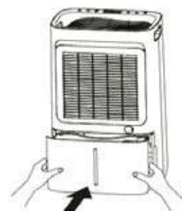
❸ Restore the water tank
