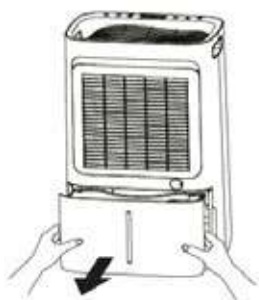
❶ Pull water tank out
